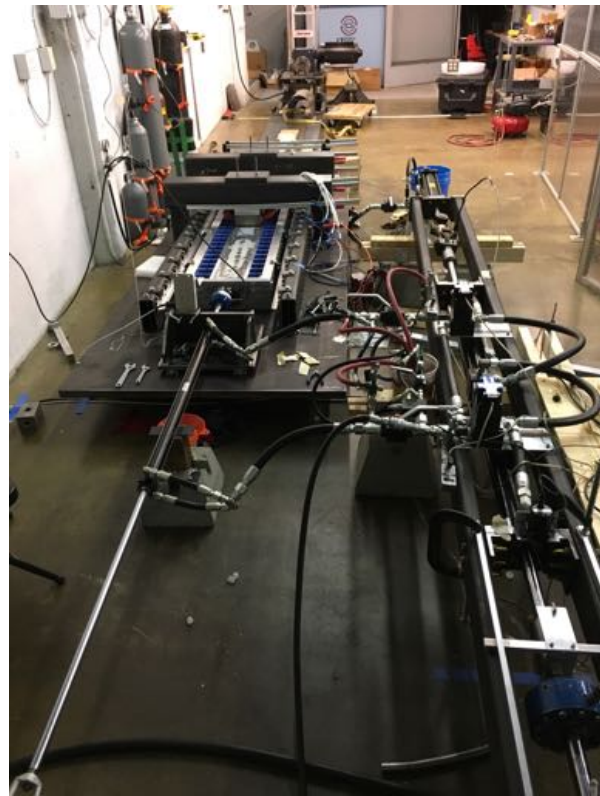
Figure 8: Laboratory test setup of the Vernier generator (left) coupled to the linear hydraulic gearbox (right). The air tanks at the top left are for the return spring
